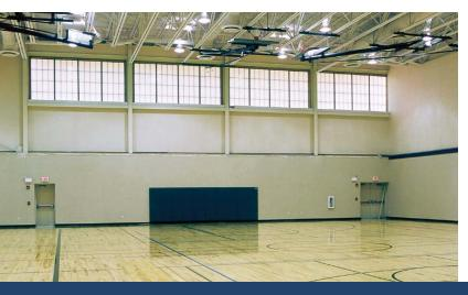
Clima-Tite™ translucent systems allow for controlled natural light to illuminate interior spaces — while eliminating glare and hot spots and reducing the need for power-hungry artificial light sources. Clima-Tite™ systems feature pultruded fiberglass support members for enhanced thermal performance, and their fiberglass reinforced face sheets significantly reduce solar heat gain. These features combine to create superior thermal performance, and assist in benefiting overall building performance.
