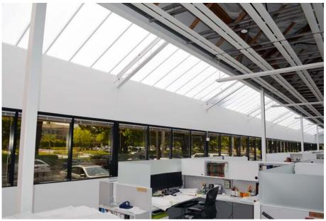
KLA replaced 9,000 sq. ft. of fiberglass skylight running the perimeter of the office building, that had yellowed and was leaking beyond repair.
