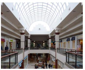
**Solution:** Fortunately, much of the existing structure remained, which helped curb the cost of the replacement. The skylight was then replaced with our Quadwall® system, which provided an even distribution of natural light that gave new life to the mall. The superior thermal and solar performance of the new skylight system also helped to better optimize building efficiency and substantially reduced utility costs.
