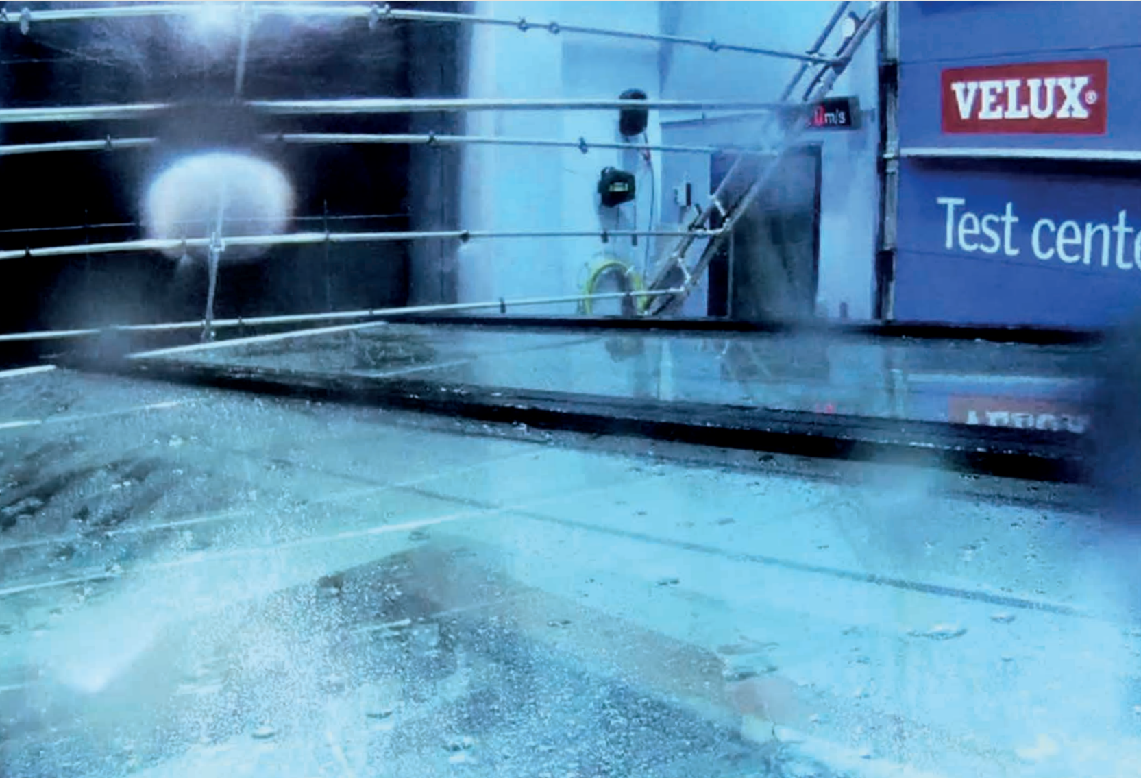
Tested in Northern Europe's largest wind tunnel with gusts reaching a full 30 M/S (storm).
